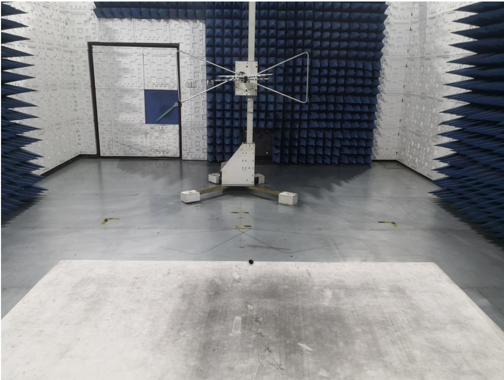
RADIATED EMISSION TEST SETUP ABOVE 1GHz
