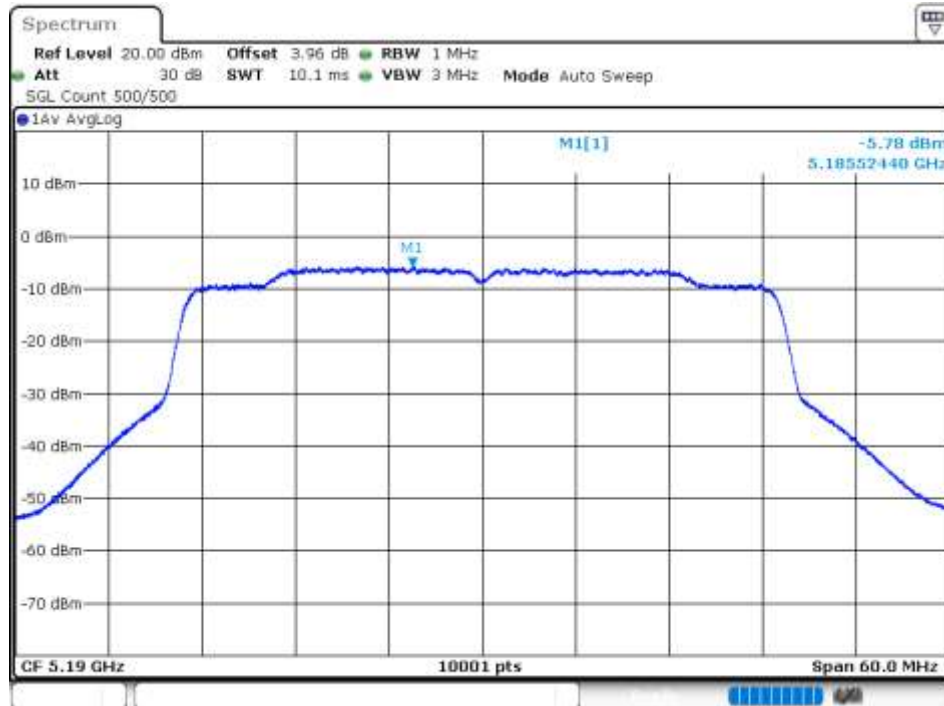
PSD NVNT ax40 5190MHz Ant1
