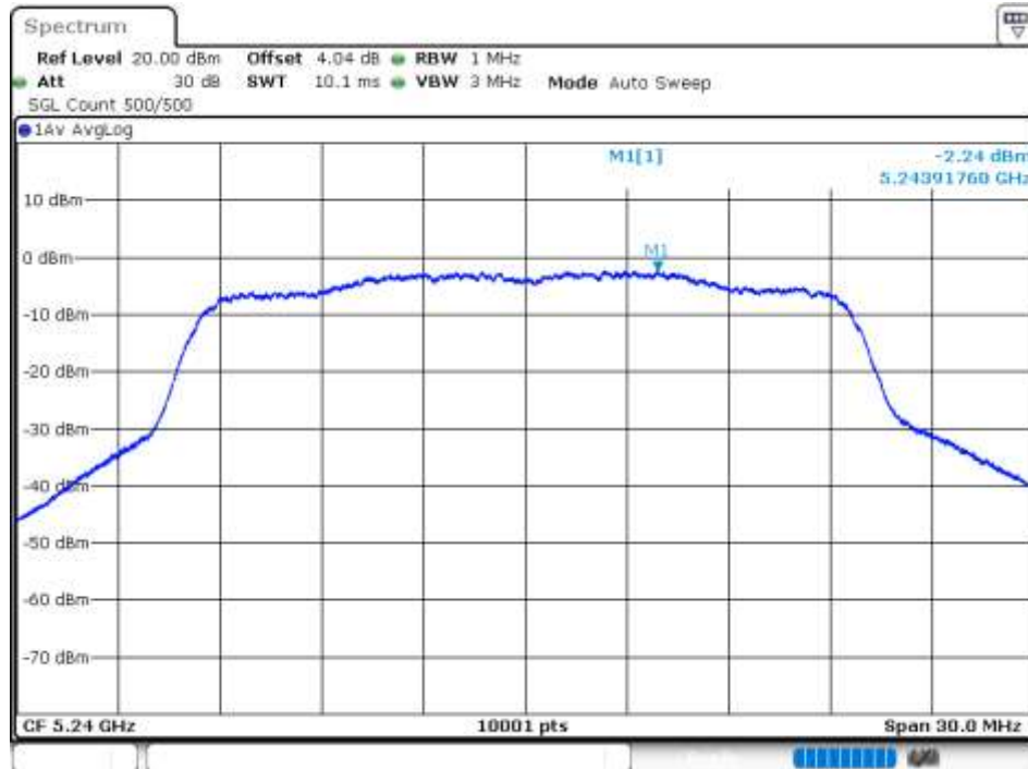
PSD NVNT ax20 5240MHz Ant1
