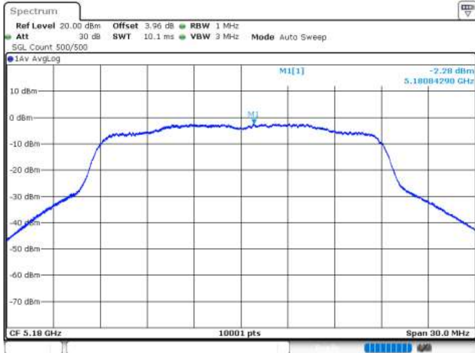
PSD NVNT n20 5180MHz Ant1
