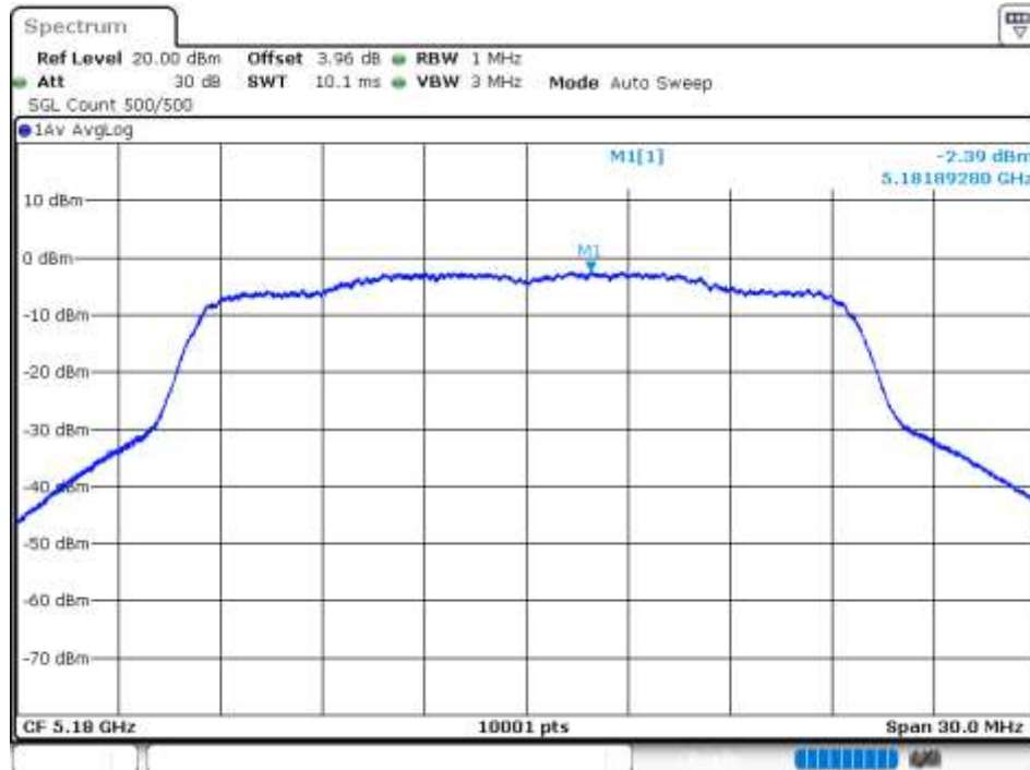
PSD NVNT ax20 5180MHz Ant1
