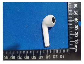
B. Top cover (B): The top cover does not provide enough physical space to fit the printing of the FCC ID according to below reference picture.
