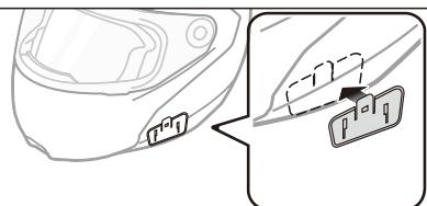
2.2) Clip-type buckle installation, find the installation position on the left edge of the helmet and clamp it, and then push it to a suitable position on the left side of the helmet.
