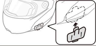
3) Align the main unit with the card slot of the buckle base and push it from top to bottom, and the installation is successful when you hear the sound of the buckle.
