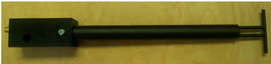
Figure 1 – MVG COMOSAR Validation Dipole
