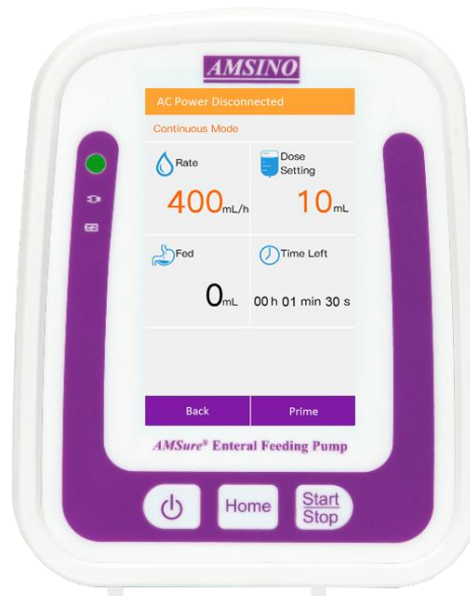
Fig 7.1.2-2 AC Power Disconnected
