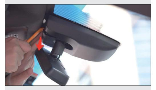
With the plastic stick we provided, pry the No.1 shell down along the direction of the red arrow.
