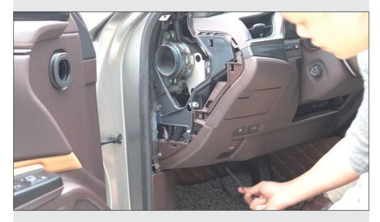
Pass the power cord up from above the floor.
