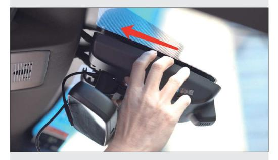
After aligning the 4 sets of matching points, push the dashcam in the direction of the red arrow. Put the machine in place.
