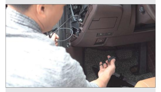
Connect the power cord to the car's OBD port. The OBD port of the car is usually above the driver's left foot.
