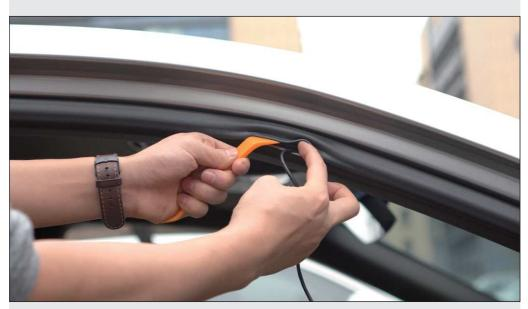
Plug the rear camera cable into the roof above the front right door.
