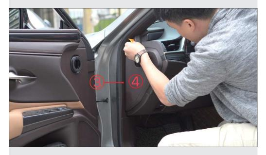
Open the left front door and remove the No.3 and No.4 shells.
