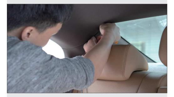
Plug the rear camera cable from the gap into the C-pillar.
