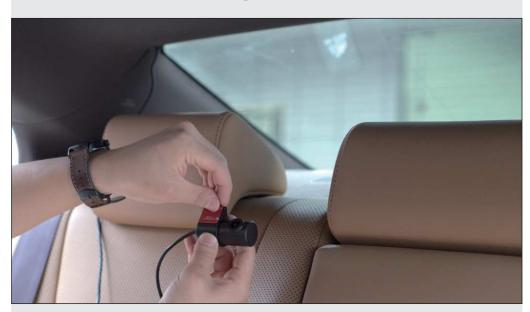
Remove the red film on the rear camera seat.
