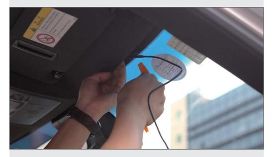
Plug the rear camera cable into the roof of the car.
