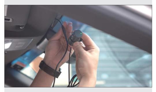
Check to see if the indicator on the rear camera is on.
