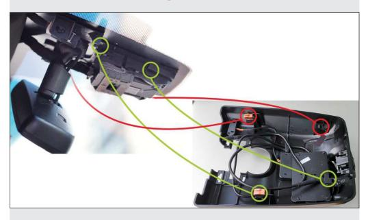
Pay attention to the 4 sets of matching points between the dashcam and the car bracket. They need to be aligned during installation.
