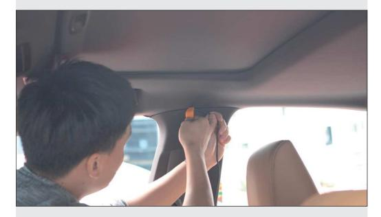
Plug the rear camera cable from the gap into the B-pillar.
