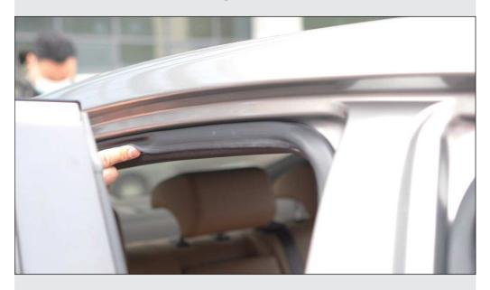
Plug the rear camera cable into the roof above the back right door.
