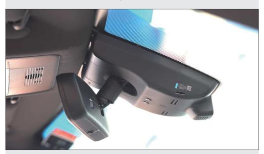
The main body of the dashcam is installed.
