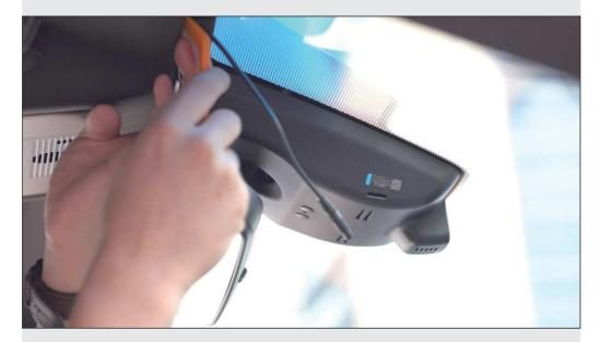
Plug the power cord into the roof on the left side of the car, and plug the rear camera cable into the roof on the right side of the car. Pay attenation to the exposed wire ends to facilitate subsequent wiring.
