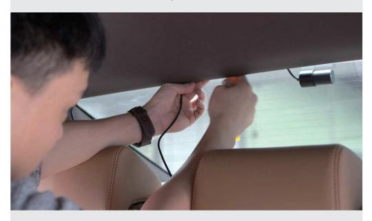
Put the extra rear camera cable into the roof of the car.
