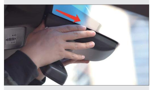
Use the thumbs of both hands to push the No. 2 shell with appropriate force in the direction of the red arrow.
