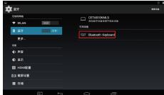
5. Enter the PIN pairing code displayed on the screen on the keyboard and press "Enter" to connect.
