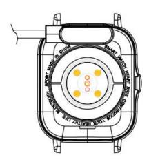
\*Please note that the two contacts of the charging cable cannot contact the conductor at the same time, which will cause the circuit to burn.
