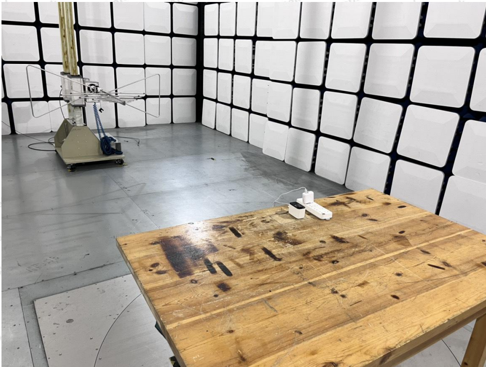
Photo of Radiation Emission Test
