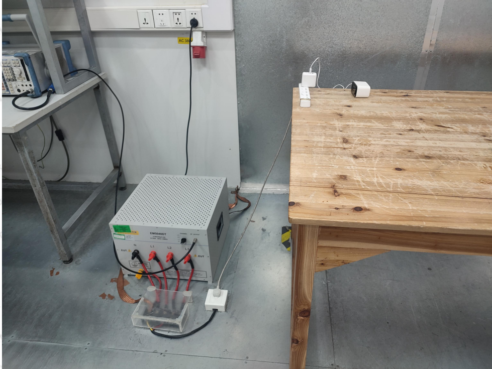
Photo of Conducted Emission Measurement
