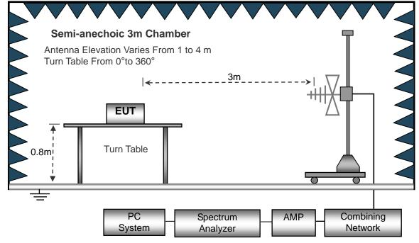
(C) Radiated Emission Test-Up Frequency Above 1GHz
