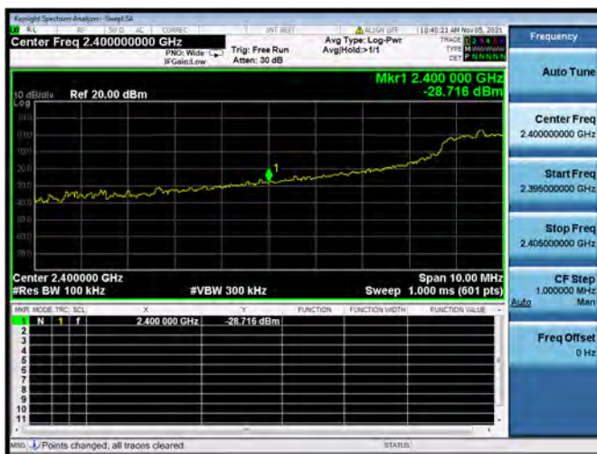
802.11g LOW CHANNEL, Carrier level
