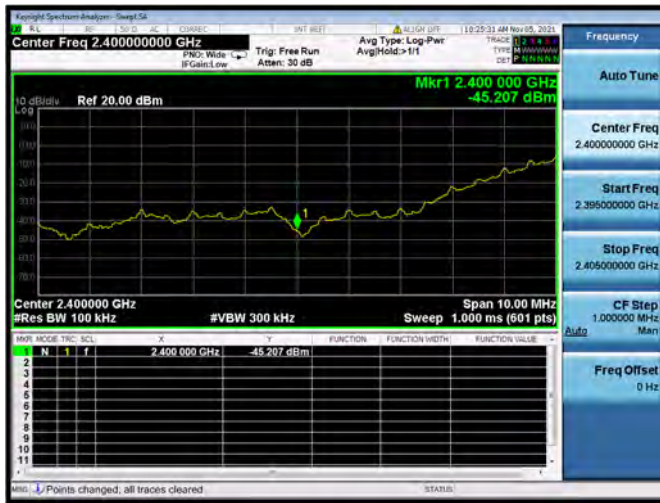
802.11b LOW CHANNEL, Carrier level
