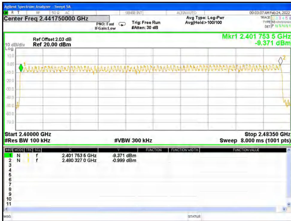
Hopping No. NVNT 3-DH1 2441MHz Ant1
