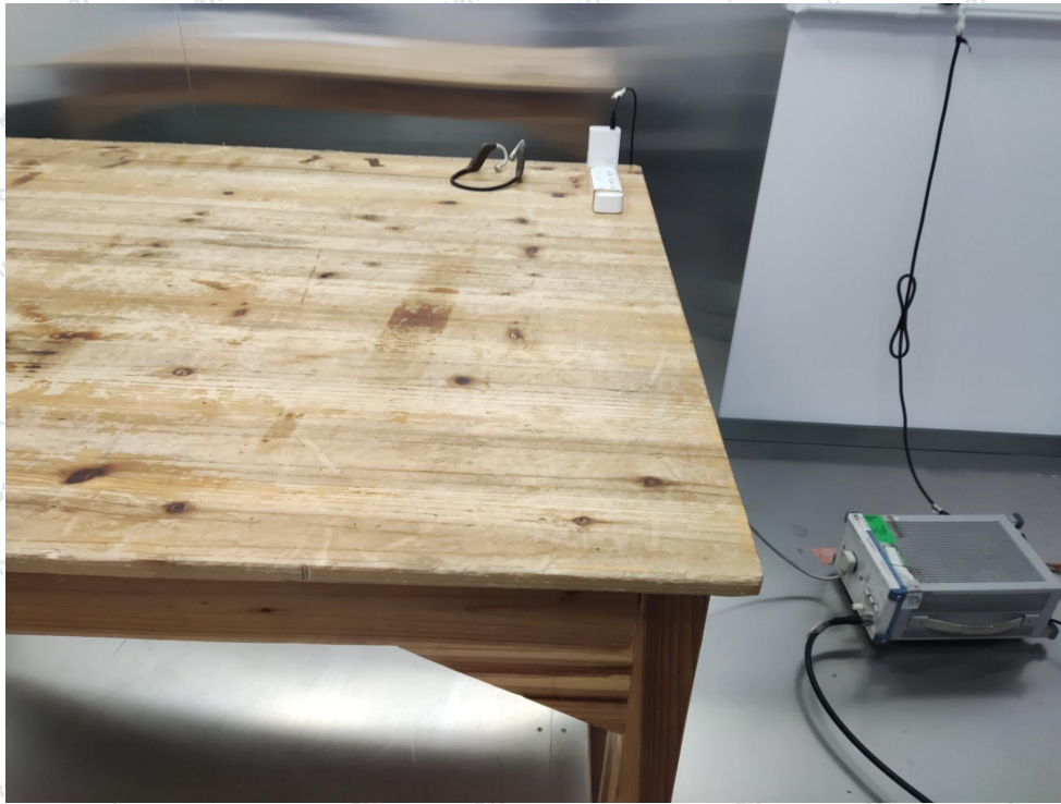
Photo of Conducted Emission Measurement
