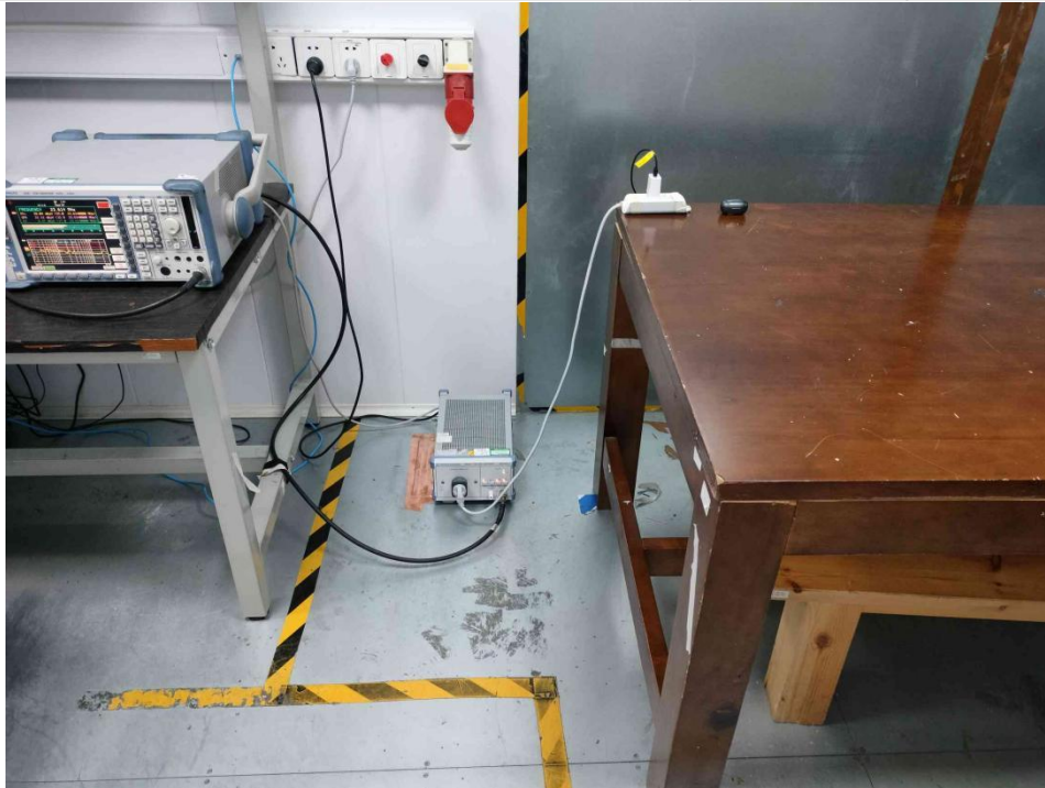
Conducted emissions at AC power line (150kHz-30MHz)
