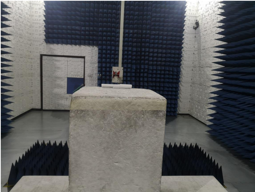
RADIATED EMISSION TEST SETUP ABOVE 1GHZ
