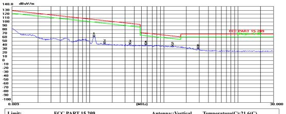
Limit: FCC PART 15.209 Antenna::Vertical Temperature(C):21.6(C) **Power Rating:** AC 120V/60Hz Humidity(%):52.7%
