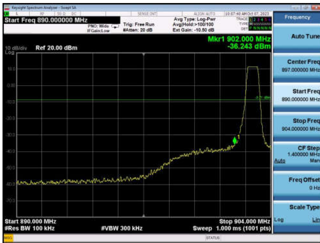
Conducted Band Edge: 903.0MHz
