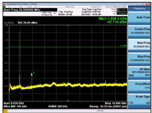
Conducted Spurious Emission: 914.2MHz
