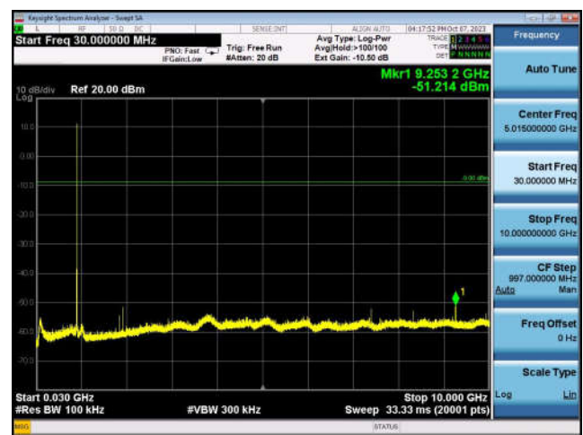
Conducted Spurious Emission: 925.1MHz
