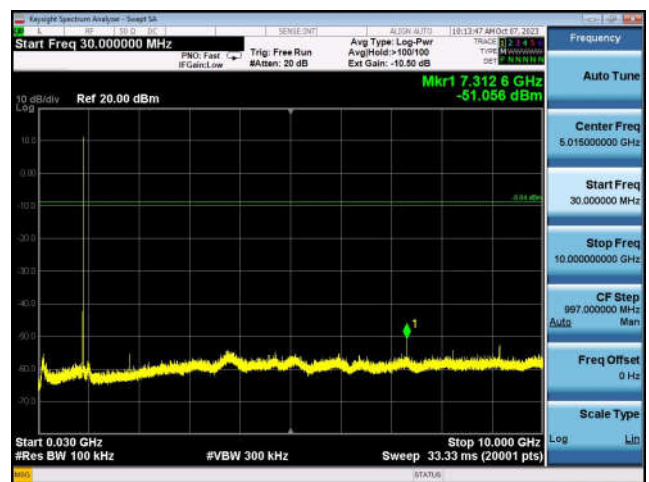
Conducted Spurious Emission: 914.2MHz
