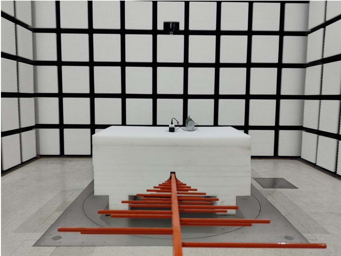
Radiated Emission Above 1GHz View
