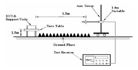
The radiated emissions were performed in the 3 meters distance, using the setup accordance with the ANSI C63.10-2013. The specification used was the FCC 15.209, and FCC 15.249 limits.
