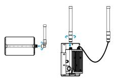
One antenna can be fixed to a pole directly via clamp kit: pass one antenna through the antenna clamp and fix it with 4 screws, then wrap the U-bolt around a pole and fix the clamp with nuts and other accessories. Besides, it can also be fixed to the short mounting backboard.
