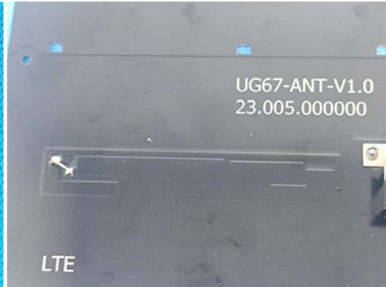
LTE Antenna (without cable, not in use)
