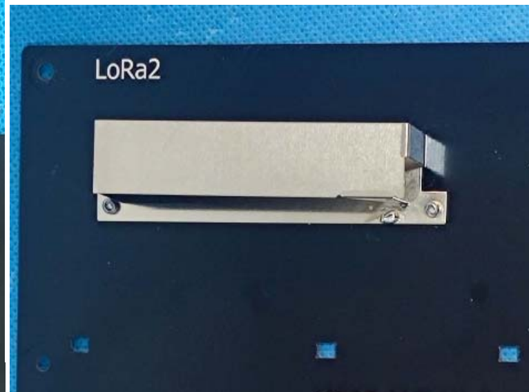
Internal LoRa Antenna 2 (without cable, not in use)
