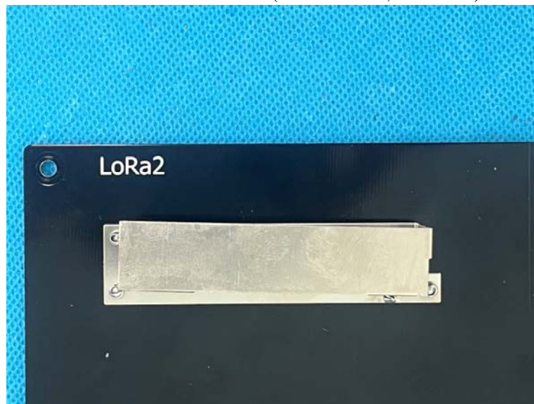
Internal LoRa Antenna 2 (without cable, not in use)
