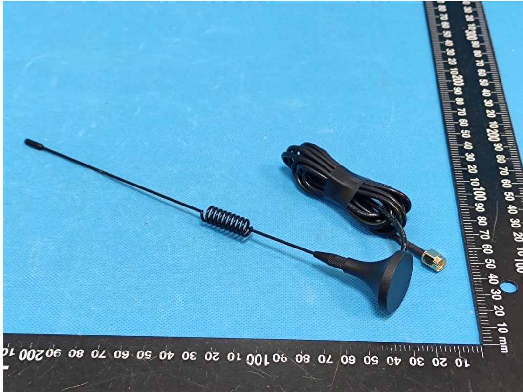
External Lora Antenna 1
