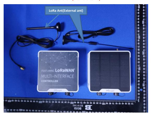
Remark: The other internal photos are totally same to UC501-915M (Internal antenna) that is shown above.
