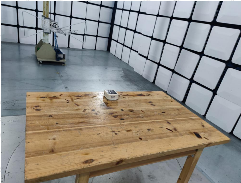
Photo of Radiation Emission Test
