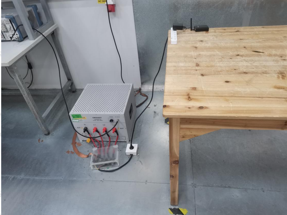
Photo of Conducted Emission Measurement
