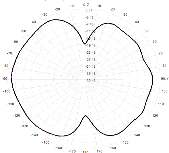
907.0MHz Total(E2-YZ), Max= -1.52dBi
