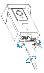
Step 4: Insert the SD Card and SIM Card.
