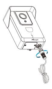
**Step 7:** Connect the device to the backplane that you've installed already and tighten the fixing screws. Then the installation is completed.
