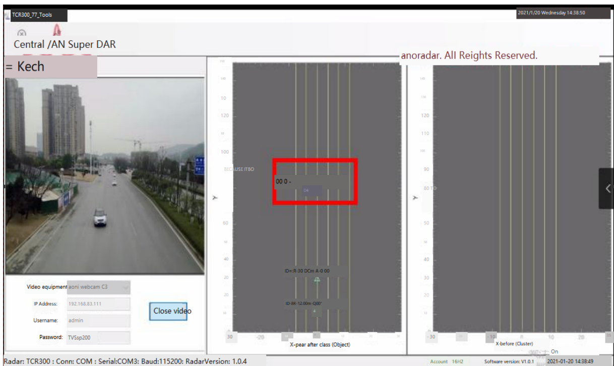
Fig. 7 Test Interface of Radar Upper Computer
