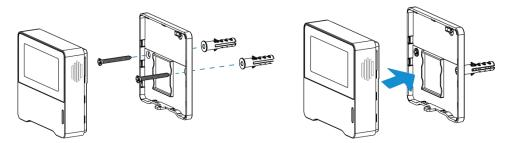
2. Fix the bottom of the device to the rear cover with the theft-deterring screw.
