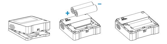
Note: The device can only be powered by ER14505 Li-SOCl<sub>2</sub> batteries not AA batteries.
