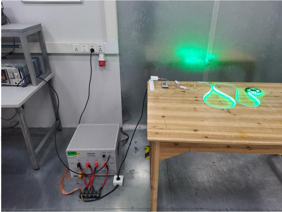
Photo of Power Line Conducted Emission Test
