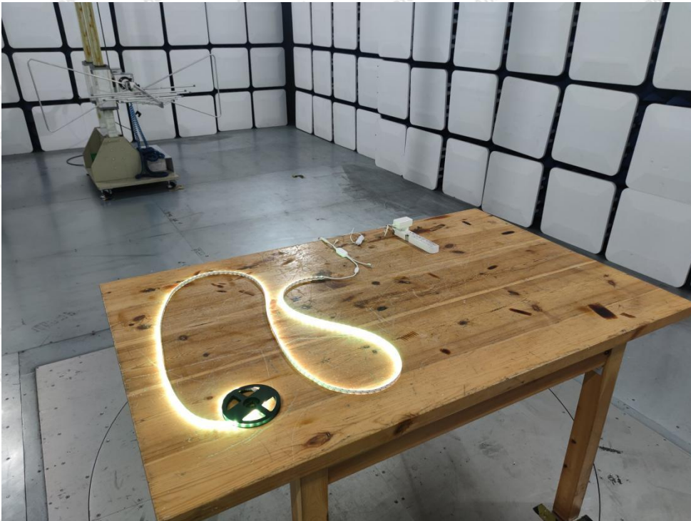
Photo of Radiation Emission Test
