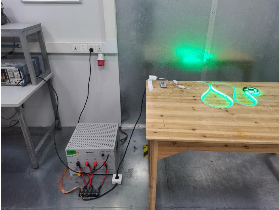
Photo of Conducted Emission Measurement
