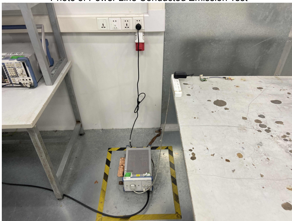
FCC ID: 2AYHW-TL8715AQ Photo of Power Line Conducted Emission Test
