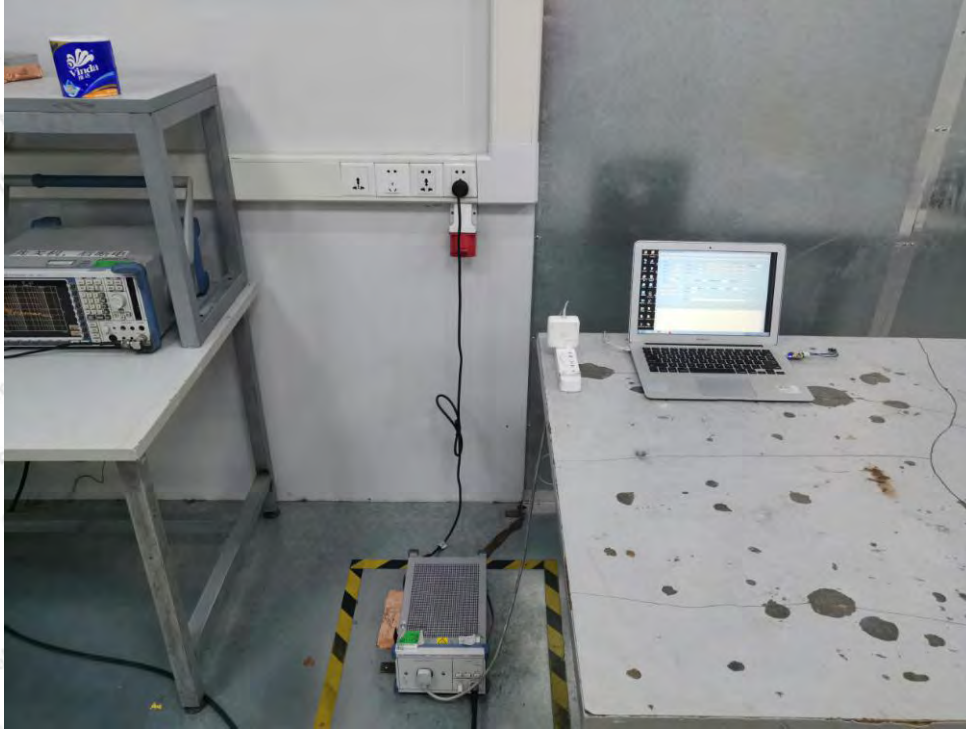
Photo of Power Line Conducted Emission Test
