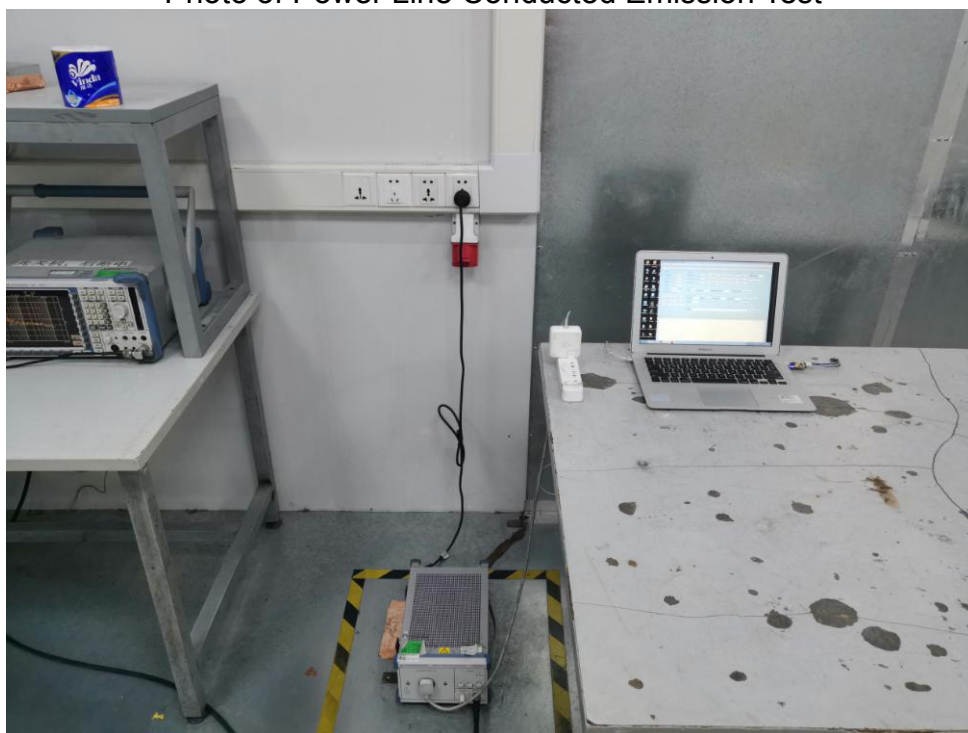
FCC ID: 2AYHW-TL7100C Photo of Power Line Conducted Emission Test
