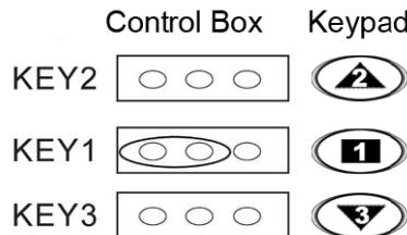
The above jumper configuration will allow
