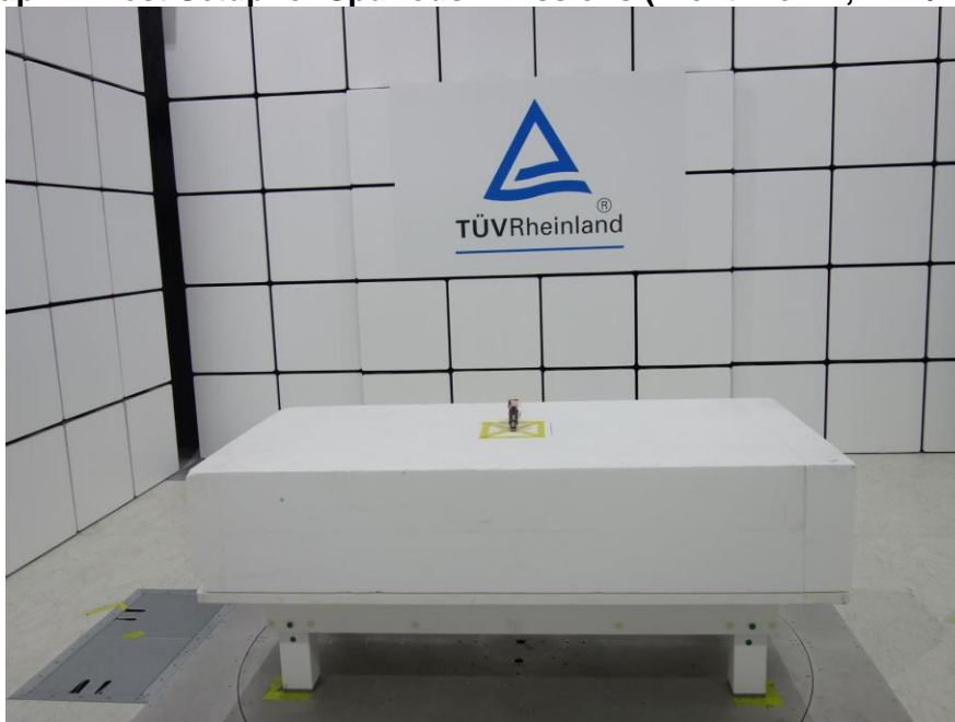
Photograph 7: Test Setup for Spurious Emissions (Front View 2, ERP/EIRP)
