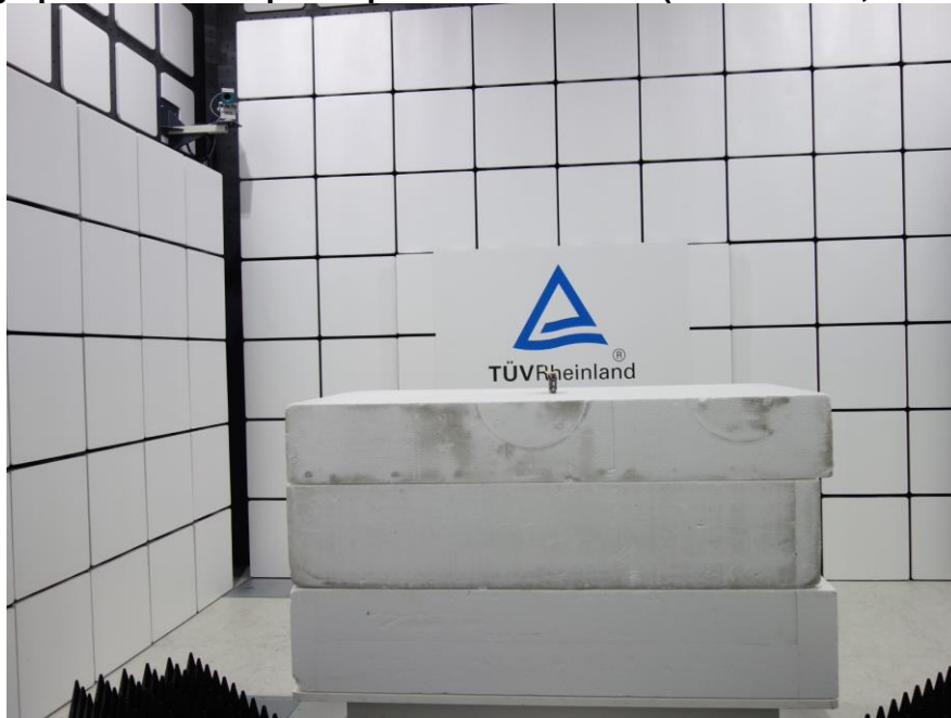
Photograph 6: Test Setup for Spurious Emissions (Front View 1, ERP/EIRP)
