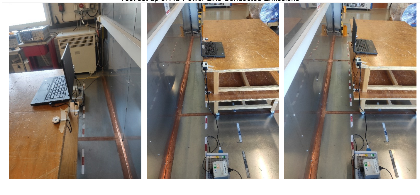
Test set up of AC Power Line Conducted Emissions
