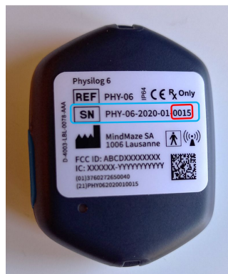
Fig 38. Physilog label with the serial number surrounded by blue and the four unique numbers to enter in the Gait Up GO mobile application surrounded by red
