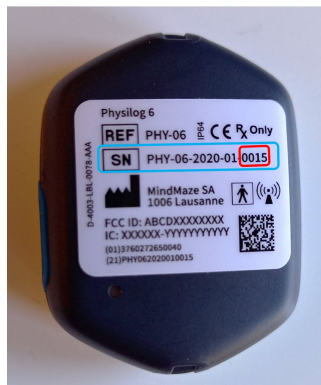
Fig 9. Physilog label with the serial number surrounded by blue and the four unique numbers to enter in the Gait Up GO mobile application surrounded by red
