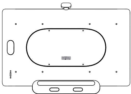
The serial number label is located on the bottom edge of the display. There you can find the link to the Meet+Avocor support page, serial number, and model information:
