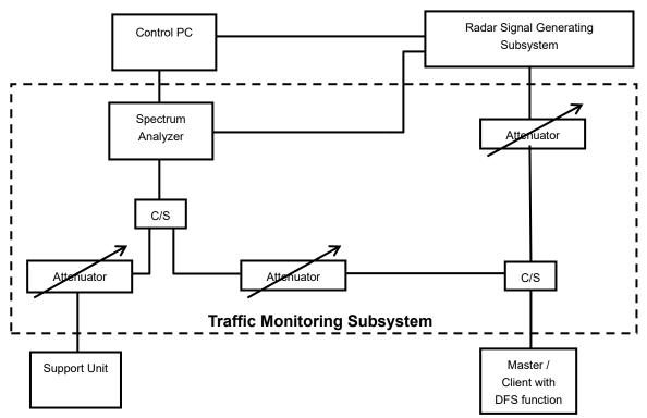
The test transmission will always be from the Master Device to the Client Device. While the Client device is set up to associate with the Master device and play the MPEG file (6  $\frac{1}{2}$  Magic Hours) from Master device, the designated MPEG test file and instructions are located at: <a href="http://ntiacsd.ntia.doc.gov/dfs/">http://ntiacsd.ntia.doc.gov/dfs/</a>.
