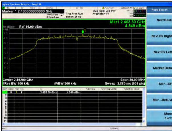
802.11n-20 MHz HIGH CHANNEL CARRIER LEVEL
