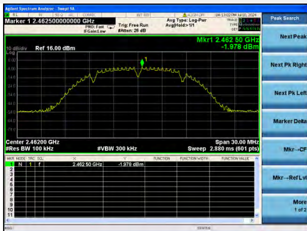
802.11b HIGH CHANNEL, CARRIER LEVEL
