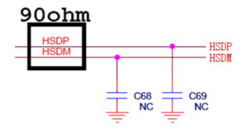
Note: USB D+/ D-differential line impedance control 90 OHM; Please reserve C68 and C69 in advance and adjust according to the actual situation.
