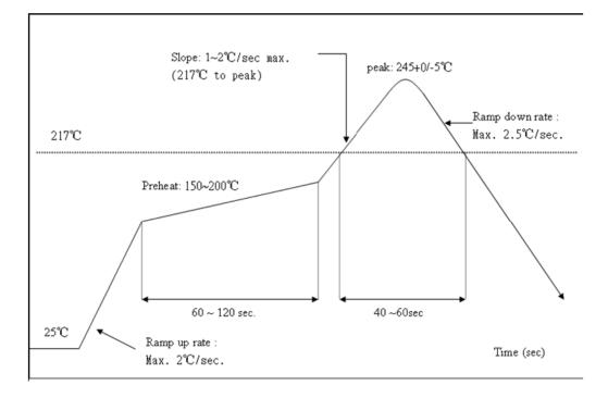
Referred to IPC/JEDEC standard. Peak Temperature : 245  $\pm5^\circ\,$  C  $\,$  Times :  $\,{\leqslant}2\,$  s
