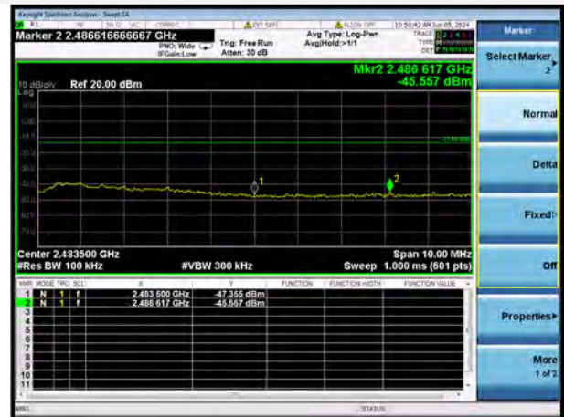
802.11b HIGH CHANNEL, BAND EDGE
