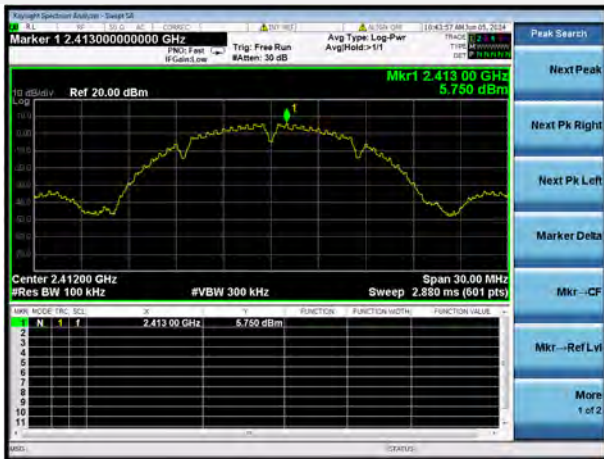
802.11b LOW CHANNEL, CARRIER LEVEL
