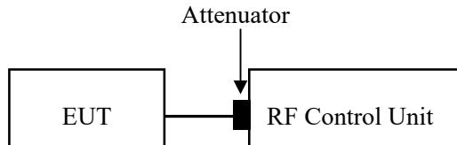
Note: the RF control unit has built-in power sensor.
