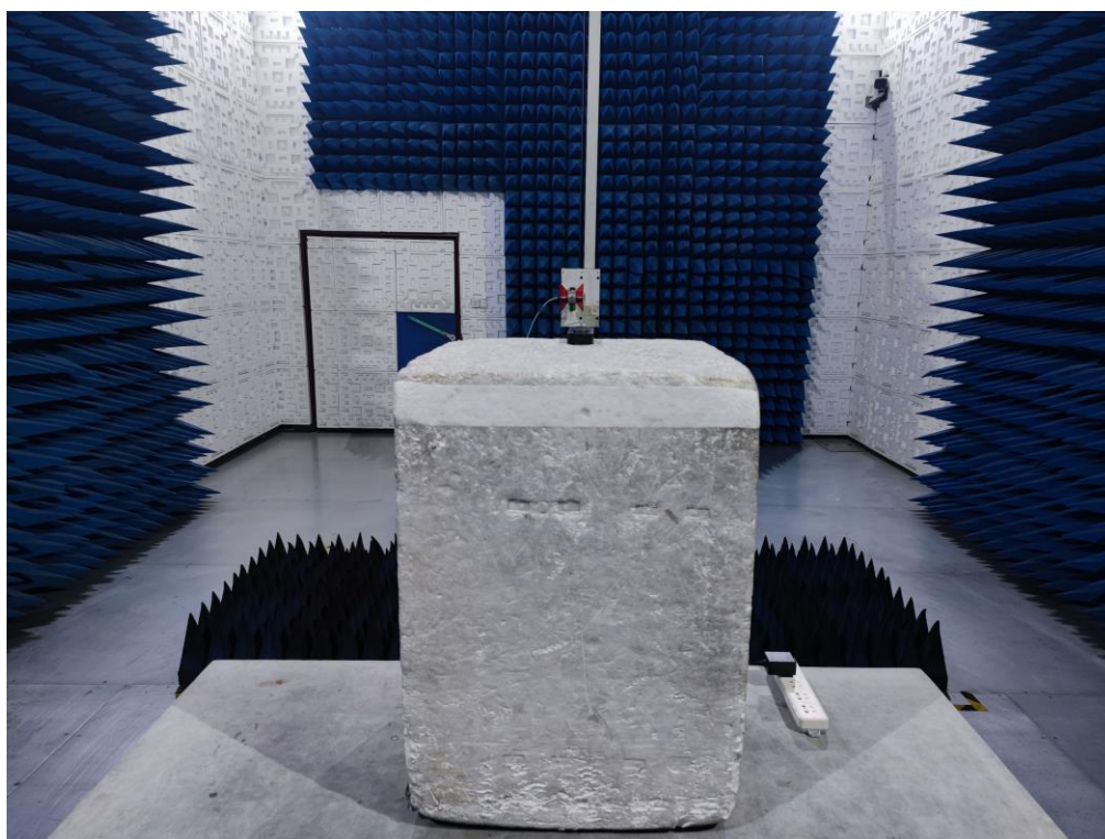
RADIATED EMISSION TEST SETUP ABOVE 1GHz
