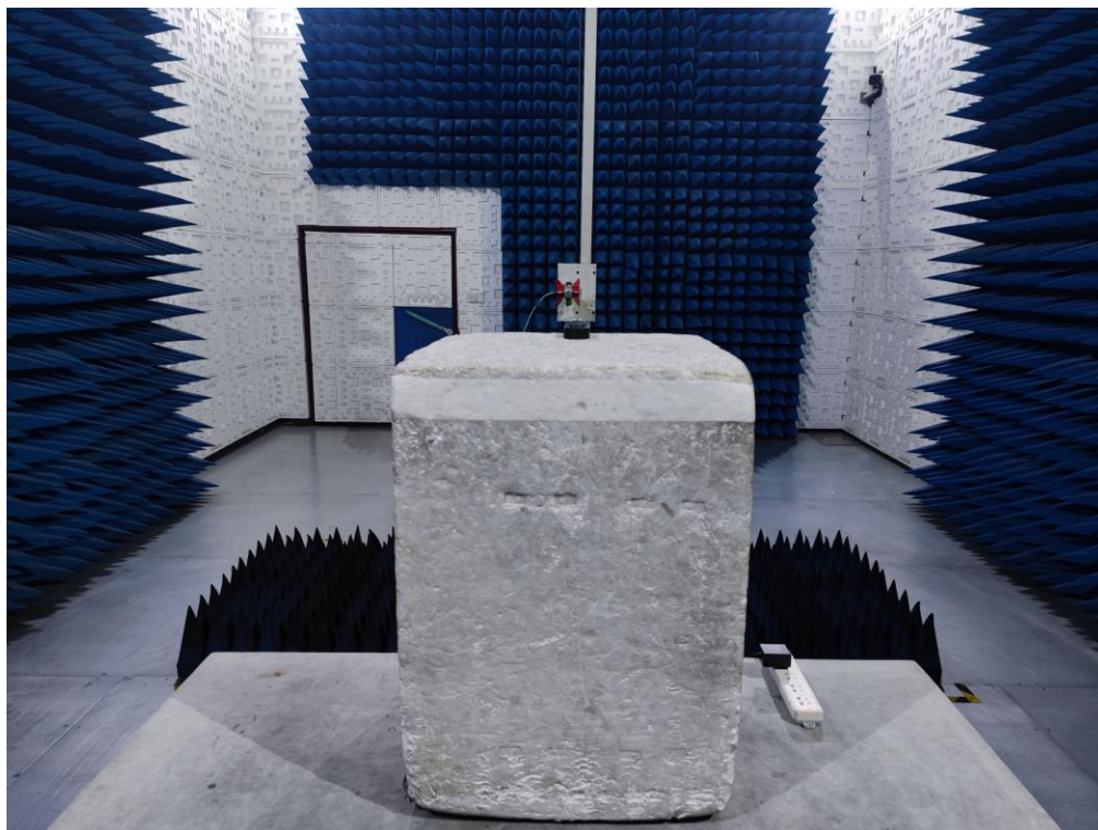
RADIATED EMISSION TEST SETUP ABOVE 1GHz
