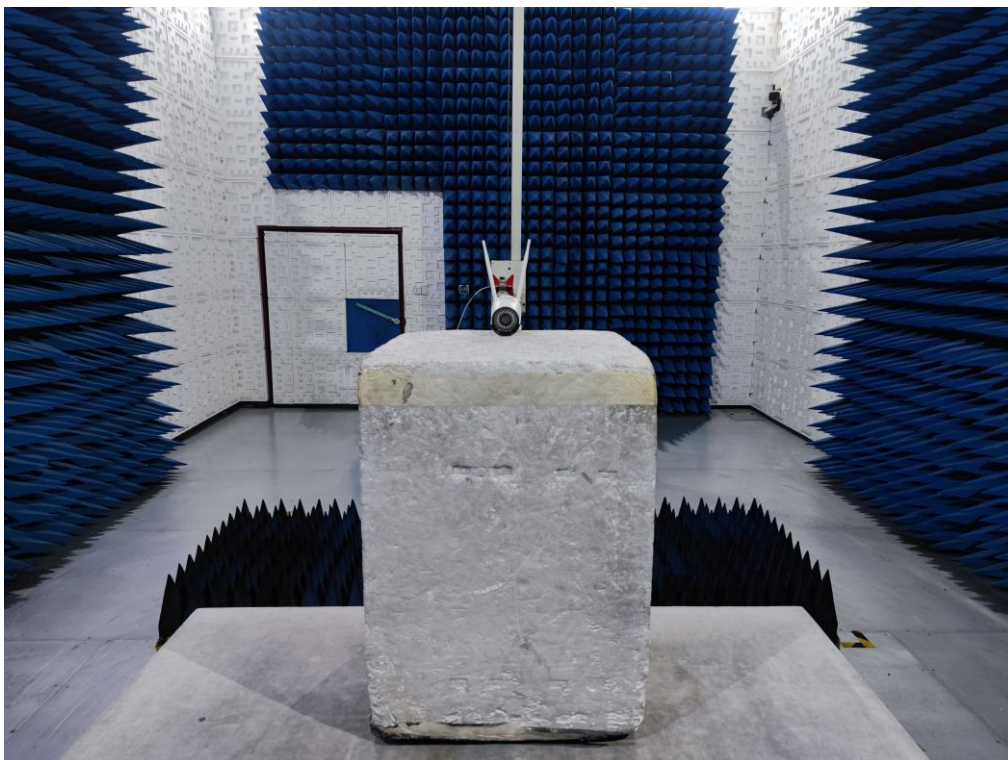
RADIATED EMISSION TEST SETUP ABOVE 1GHz
