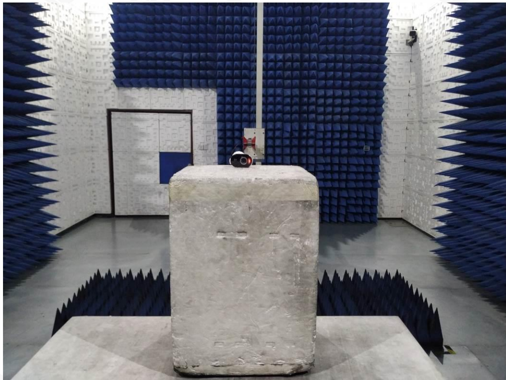
FCC RADIATED EMISSION TEST SETUP ABOVE 1GHZ
