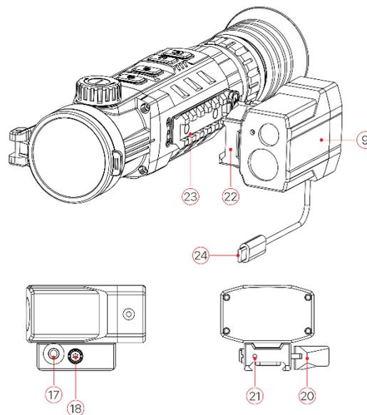
➤ Then tighten the lock screw (21) on the back of the mount with a hex-nut wrench.
