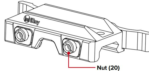
2. Move the lever to the open position. This will make the adjustment nut protrude on the opposite side of the base.
